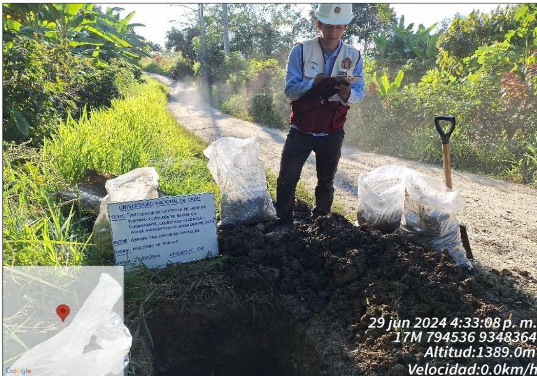
**Figura 40***Muestreo de suelos en la calicata N° 01.*
