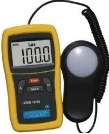
The image shows a yellow Victor 1010A luxometer with a black spherical sensor on a cable. The LCD screen displays '1000' Lux. The device has buttons for 'ON/OFF', 'MAX', and 'A'. The text 'VICTOR 1010A' and 'AUTO DIGITAL LUXMETER' are visible on the front panel.
